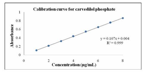
Figure 2. Calibration curve for carvedilol phosphate.
