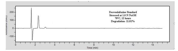
Figure 4. Chromatogram of desvenlafaxine, stressed in 1.0 N NaOH at 70°C for 12 hours.
