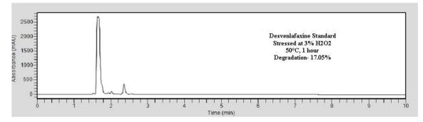
Figure 5. Chromatogram of desvenlafaxine, stressed in 3  $\%~H_2O_2$  at 50°C for 2 hours.
