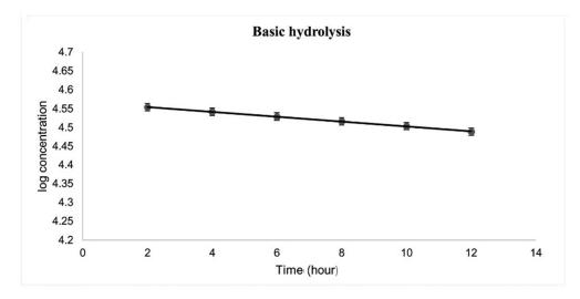
Figure 8. Desvenlafaxine degradation kinetics at 70°C under 1.0 N NaOH stressed conditions.
