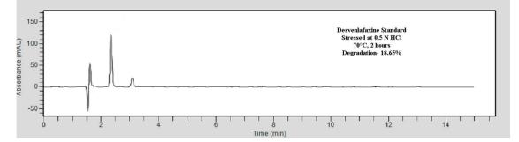
Figure 3. Chromatogram of desvenlafaxine, stressed in 0.5 N HCl at 70°C for 2 hours.
