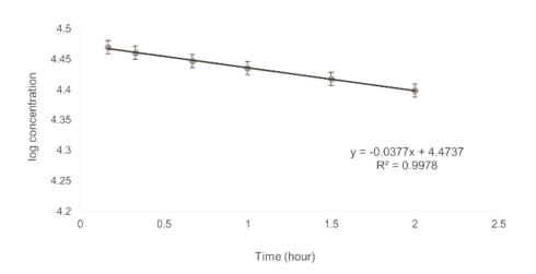
Figure 7. Desvenlafaxine degradation kinetics at 70°C under 0.5 N HCl stressed conditions.
