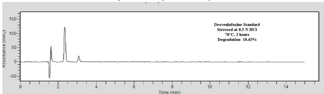
Figure 3. Chromatogram of desvenlafaxine, stressed in 0.5 N HCl at 70°C for 2 hours.
