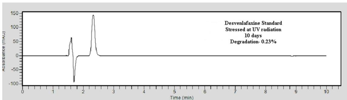
Figure 6. Chromatogram of desvenlafaxine, stressed in UV light for 10 days.
