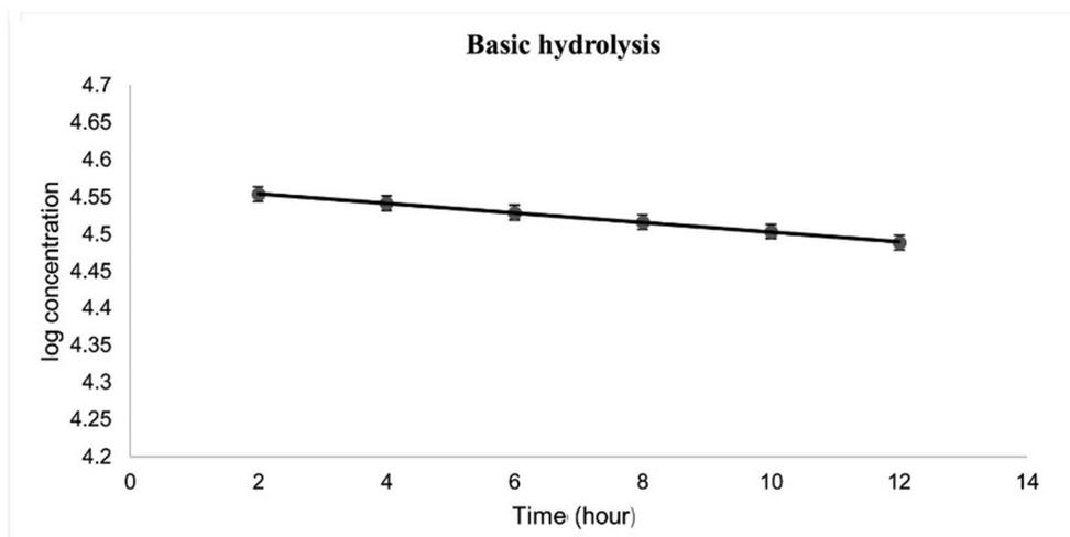
Figure 8. Desvenlafaxine degradation kinetics at 70°C under 1.0 N NaOH stressed conditions.
