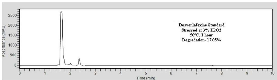
Figure 5. Chromatogram of desvenlafaxine, stressed in 3 % H<sub>2</sub>O<sub>2</sub> at 50°C for 2 hours.
