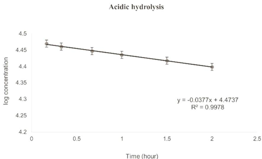
Figure 7. Desvenlafaxine degradation kinetics at 70°C under 0.5 N HCl stressed conditions.
