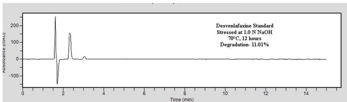
Figure 4. Chromatogram of desvenlafaxine, stressed in 1.0 N NaOH at 70°C for 12 hours.
